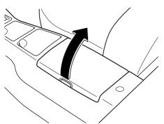
The center console has a lockable lid, insert the key into the slot; then turn the key clockwise to lock, counterclockwise to unlock.
