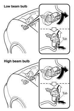
5. Install the new bulb in the reverse order of removal.
