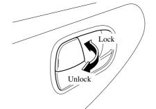
To lock any door with the door-lock button from the outside, push its doorlock button and close the door.
