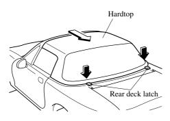
8. Lift the hardtop straight off the body to prevent damage to the rear deck latches and studs.
