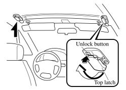
6. Lift up on the front section of the top to release it from the windshield header.
