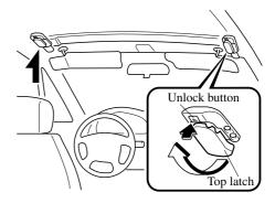
5. Push the unlock buttons and fully release the side latches.
