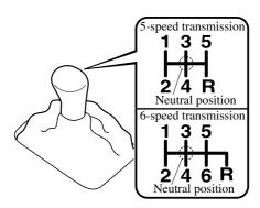
The shift pattern of the transmission is conventional, as shown.
