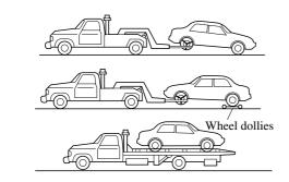
If the transmission, rear axle, and steering system are not damaged, the vehicle may be towed on all four wheels. If any of these components are damaged, use wheel dollies or flatbed equipment.
