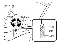
The level must be kept between the H and L marks.
