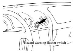
Depress the hazard warning switch and all four turn signals will flash at once.
