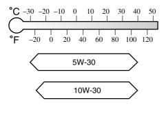
When choosing an oil, consider the temperature range your vehicle will operate in before the next oil change. Then select the recommended viscosity from this chart.
